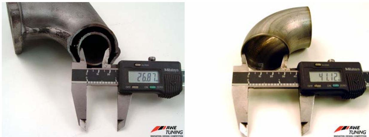
Figure 5: Comparison of secondary runner diameters. Stock is pictured on the left, AWE Tuning on the right. The AWE Tuning secondary runner is ~50% larger than stock, which is appropriate given the proportional increase of gas volume in this area of the manifold. The stock secondary diameter is the same as the primary diameters!
