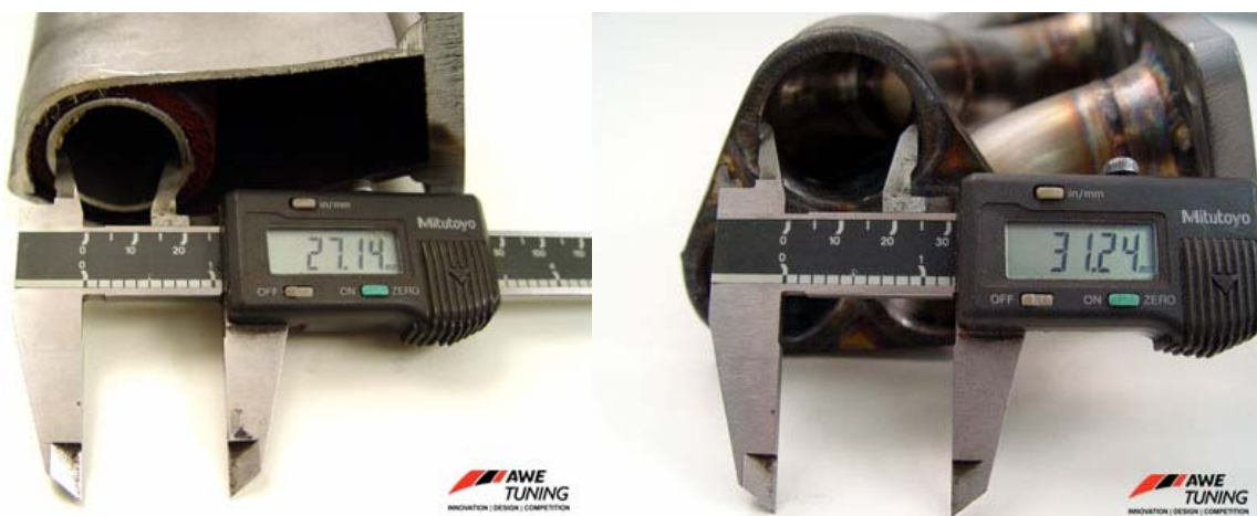
Figure 4: Comparison of primary runner diameters. Stock is pictured on the left, AWE Tuning on the right. The AWE Tuning primary runners are only 15% larger than stock, which is sufficient for ~475hp on the 2.7T when mated to a proper collector design.
