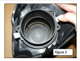
Install the AWE air filter into the airbox lid by lining up the rubber bosses on the filter with the openings in the airbox lid.
