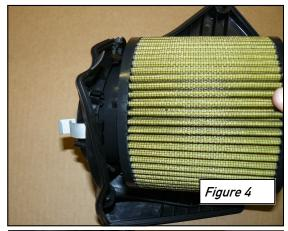
Use the supplied M4 bolts to secure the filter to the lid.
